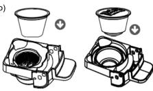
3 Insert the Adapter into the machine, make sure you put it into the end, then close the Handle.
